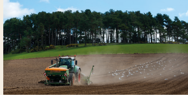
Tractor pulling a 'One Pass' which will sow the seed, plant fertiliser, harrow the soil all in one pass.
